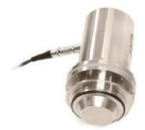
The Compact Yeast Monitor measures the concentration of live yeast on-lineThe Compact Yeast Monitor is designed to be fitted on to standard instrument housings such as the Tuchenhagen varivent. This robust instrument is completly contained within an IP65 staineless steel housing.
